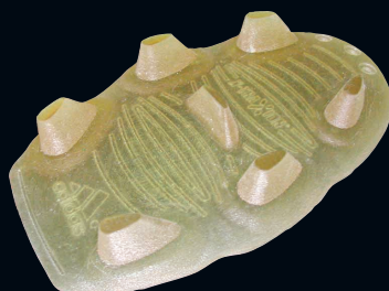
3D Part with Support Structure Removed
