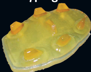
Objet Printed Part with Support Structure
