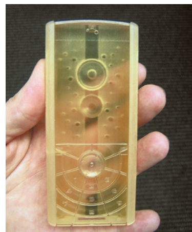
Model printed on an Eden 3-D printing system.
