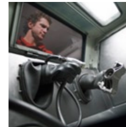
The Arcam Powder Recovery System in action.
